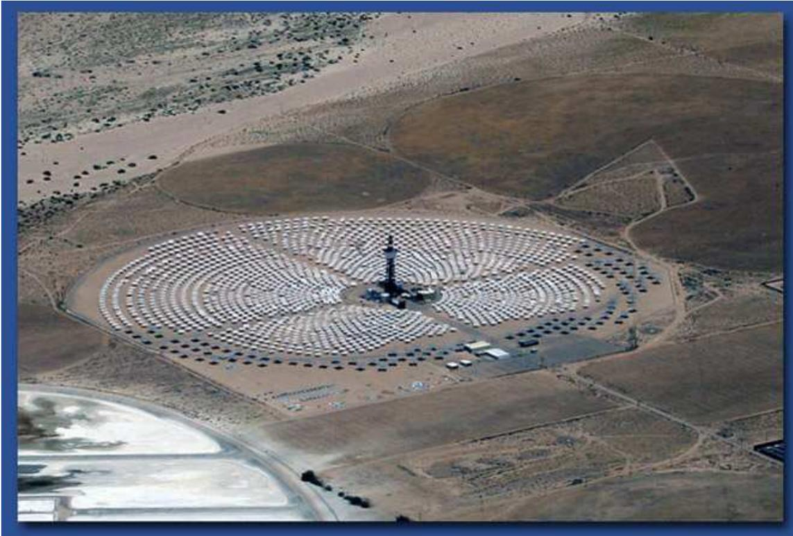
When completed, the Ivanpah Solar Electric Generating System will have gross capacity of 392 megawatts. Not bad.
